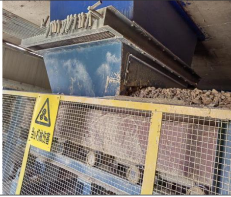
破碎、下料口等产尘点均配套集气罩，布袋除尘器等
