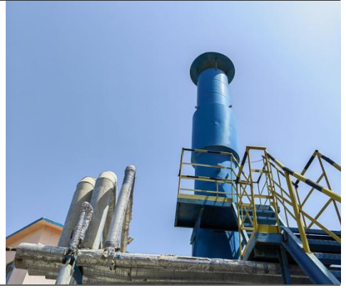
破碎、下料口等产尘点均配套集气罩，布袋除尘器等
